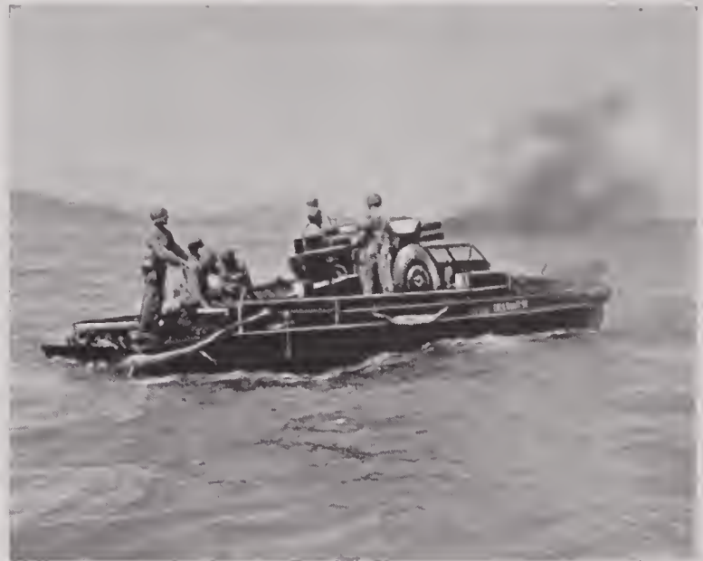
FIGURE 88. 105-mm howitzer on DUKW can also be fired at sea.
